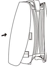
5 Restore the filter screen on the left side: hang the upper part of the filter screen and then lightly tug in and fasten the lower part.
