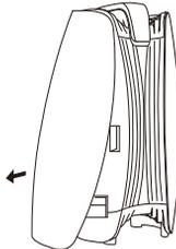
2 Remove the filter screen cover on the left side of the product and pull out the filter screen from the middle position in the lower part of the cover.
