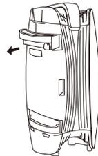
3 Pull out and remove the filter screen drawer
