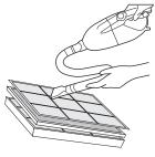
6 Clean or replace the filter with a vacuum cleaner (Pre Filter can be washed with water and dried before
