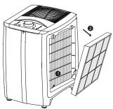
Slide the HEPA along the slot and remove it by lifting it outwards
