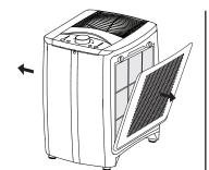
Open the filter covers on both sides: pull out the filter covers on both sides in the upper part of the product.
