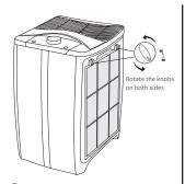
4 Rotate the Fixing knob
