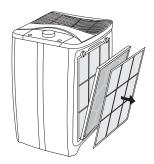
Take out the primary filters and Molecular filters (remove the plastic bags of new filters)
