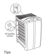
In order to better use the air cleaner, do not block the openings of the smell sensor, or the dust sensor on the strip behind the machine. Often clean them and keep them clean.
