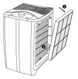
Lift the Main filters outward and take it out along the chutes on both sides
