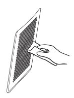
After the filter cover is removed, use the vacuum clean small brush or a wet cloth to gently wipe the filter cover, wait it to dry, and then fit it back into the machine.
