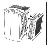
Put the filters back in order, and cover the filter covers.
